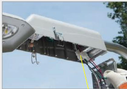
Hinged, Removable Power Door Driver is mounted to door. Integral hinge allows door to hang securely while making wire connections and can be easily removed without the use of tools.
