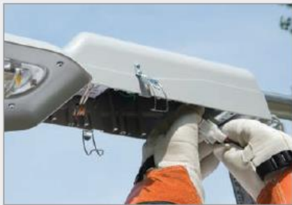
Hinged, Removable Power Door Driver is mounted to door. Integral hinge allows door to hang securely while making wire connections and can be easily removed without the use of tools.
